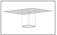
2. Attach to ceiling using expansion screws provided.
