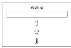
1. Drill pilot holes in mounting surface. Install expansion screws and connectors.
