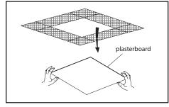
1. Power off before installation and ensure installed object can bear fixture weight. Open groove on ceiling according to corresponding size. Install fixture into clamping groove on ceiling. Drill holes.
