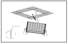
3 Insert DC male head into DC female head and finish installation.
