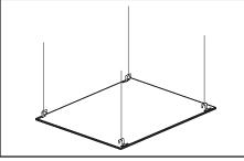
2. Attach cables to earthquake clips found on back of luminaire.
