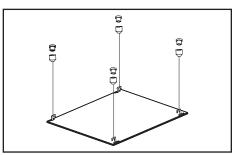
3. Attach other end of cable to connectors mounted in ceiling.
