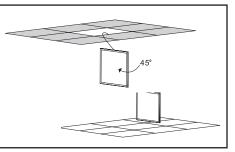
2. Rotate luminaire by 45° and pass through ceiling.
