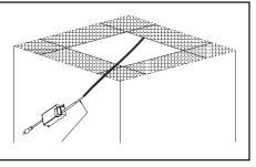
2. Connect wire attached to fixture to corresponding power cord and carry out insulation sealing at joint. Brown wire connects with L and Blue wire.
